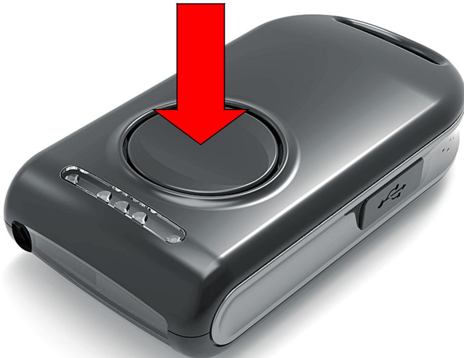
You will head two beep sounds. Release the button. Now the scanner is in pairing mode and can be browsed from the PDA, smart phone or a PC.
